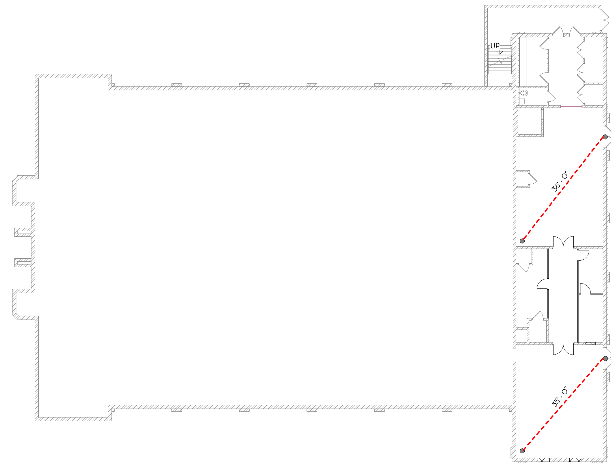
6 BASEMENT LIFE SAFETY PLAN - TRAVEL DISTANCE 1/16" = 1'-0"
