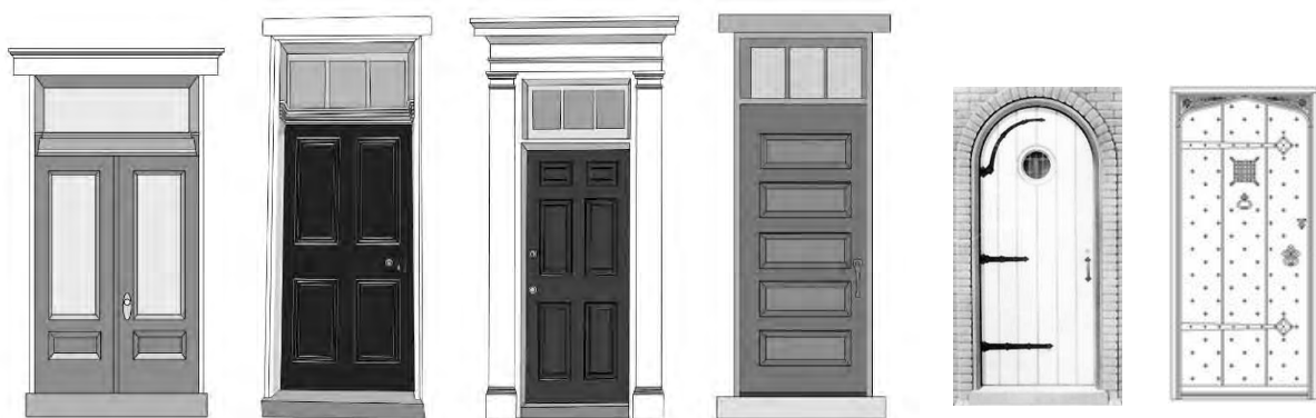
Illustration 16: Paneled doors throughout the district are evident in a number of configurations. A panel at the base of a door is common in single and double doors. The four- and six- panel doors are the most common doors, and the five-panel door usually indicates twentieth century construction or a replacement door.
