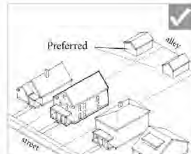
To the extent plainly visible from the street, the tradition of detached secondary structures is encouraged because this reduces the overall perceived mass of buildings on the site.
