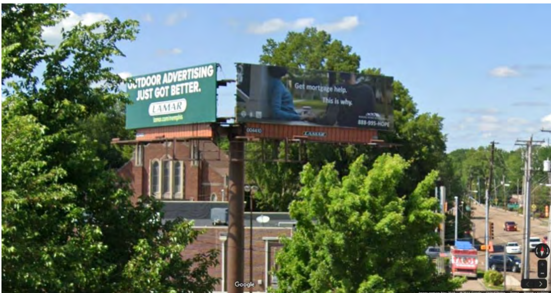
Example of a sign at Sam Cooper and Highland with a splay of 90 degrees, which allows both signs to be read at the same time.
